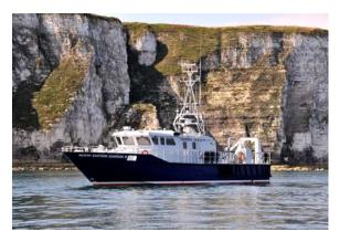
The North Eastern Guardian III (NEG III) is a 26m-patrol boat, (built and delivered November 2007), capable of a top speed of 26 knots and equipped with the latest electronic navigation systems and marine survey and monitoring equipment.
