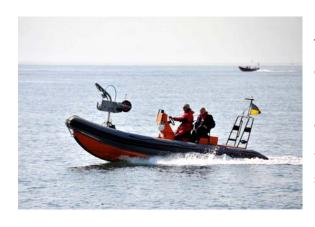
The NEGIII carries a 6.4 metre RIB capable of speeds up to 30 knots. The RIB is primarily used for supporting offshore enforcement operations, but is also available to support scientific survey work, such as side scan sonar.
